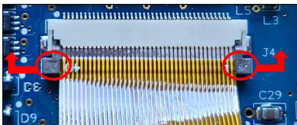
To remove the ribbon cable, lift up the two tabs on both ends. This will loosen the ribbon cable so it can be pulled out.
