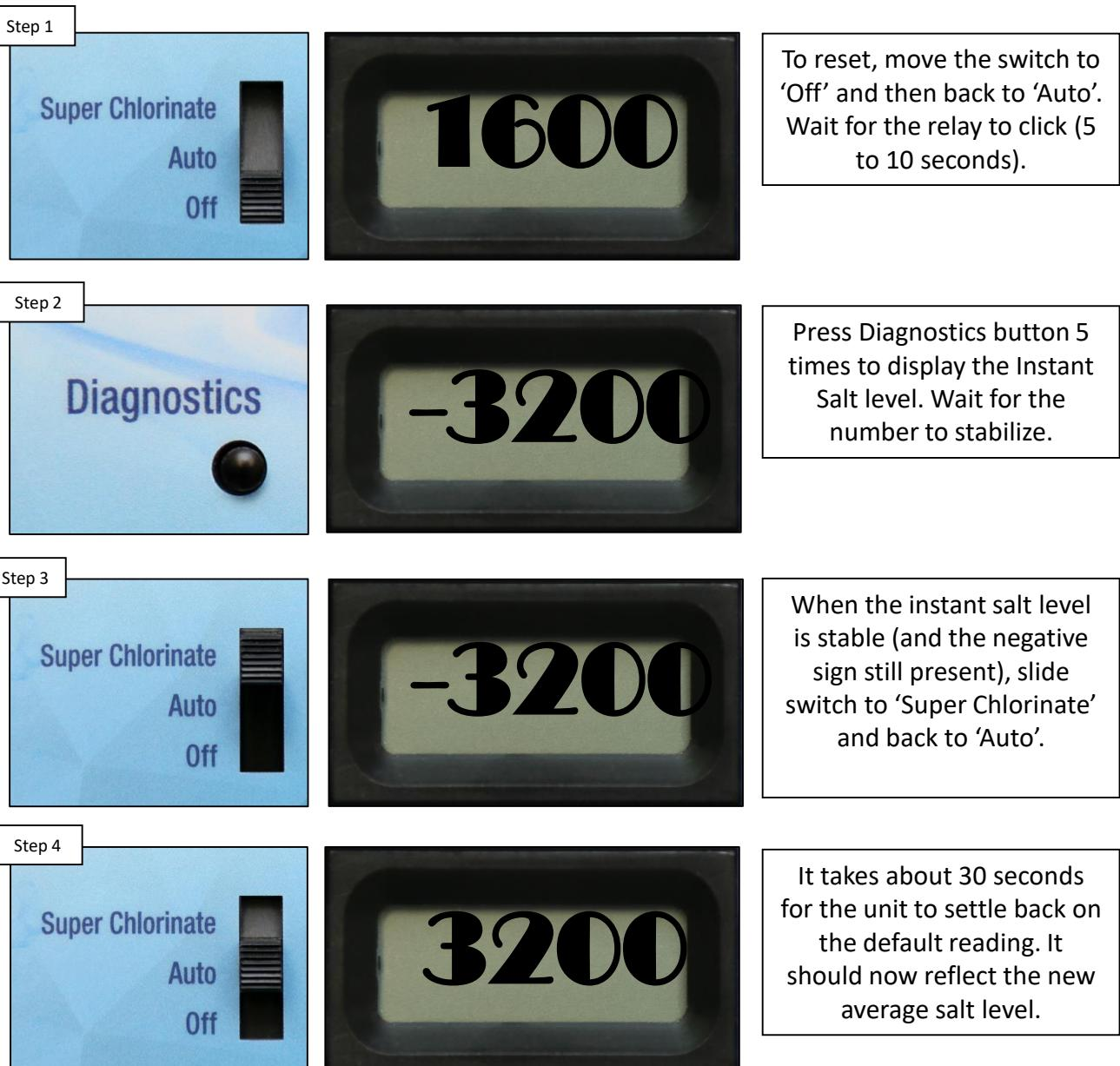
**NOTE:** Repeat this process once more to ensure both polarities are reading within 500ppm of each other.
