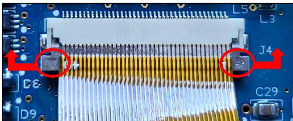
To remove the ribbon cable, lift up the two tabs on both ends. This will loosen the ribbon cable so it can be pulled out.
