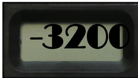
Press Diagnostics button 5 times to display the Instant Salt level. Wait for the number to stabilize.
