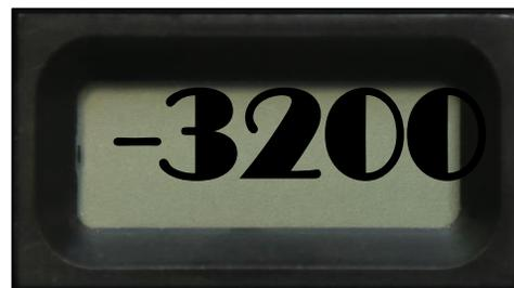
When the instant salt level is stable (and the negative sign still present), slide switch to 'Super Chlorinate' and back to 'Auto'.
