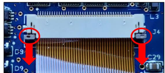
To remove the ribbon cable, pull down on the two tabs on both ends. This will loosen the ribbon cable so it can be pulled out.
