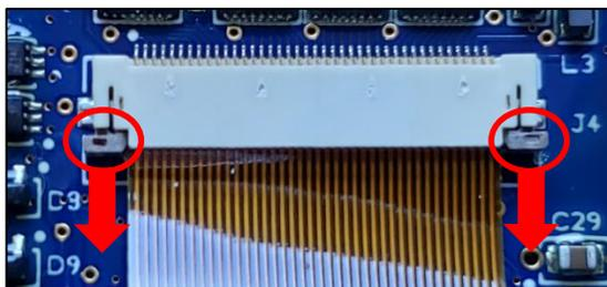
To remove the ribbon cable, pull down on the two tabs on both ends. This will loosen the ribbon cable so it can be pulled out.
